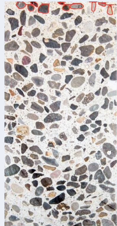
Figure 2: SCC samples based on AALBORG WHITE®. Left: unadjusted mix (1:1 replacement of grey cement with AALBORG WHITE®), right: same mix, after adjustment. Images of final flow spread shown above. Segregation calculated according to the procedure is respectively 3.2% and 0.7% for the two samples.
